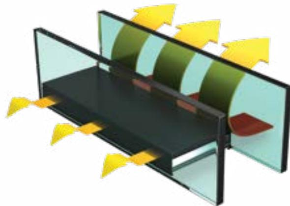
The Duralite® spacer is a component laminate design that optimizes the use of a number of spacer components. All spacers need adhesives, sealants, structural elements and desiccant to perform. They also need to last a long time under adverse conditions inside your window frame. Duralite is designed to seal your window better and longer, while increasing energy savings compared to other types of spacers.
