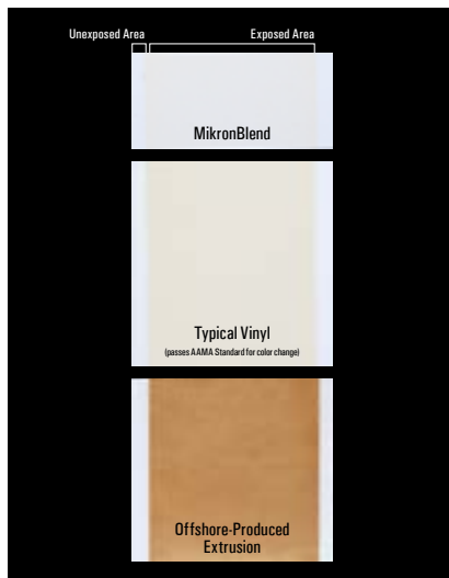
Actual, unaltered photo of samples after 1 year equivalent UV accelerated weathering via Xenon-Arc.
