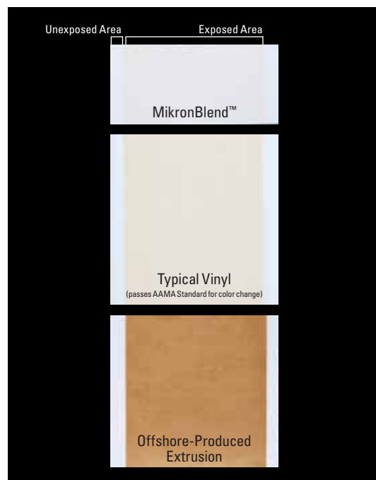
Actual, unaltered photo of samples after 1 year equivalent UV accelerated weathering Xenon-Arc.
